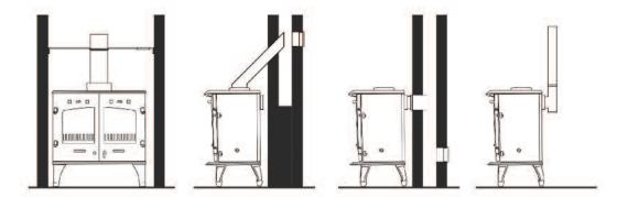
Attach the flue outlet to the stove with the screws and nuts provided. Use a steel closure plate to seal off the chimney; a cleaning door must be fitted into the plate or flue, and a steel sealing collar must be used to fit the flue into the steel plate. Seal all joins with fire cement.
