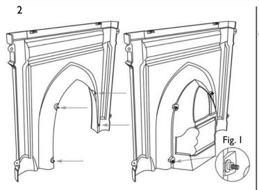
Insert the 4 M6 Studs into the back of the Fireplace Fascia. Attach Fireplace Back to the back of the Fireplace Fascia, ensuring that the M6 Studs pass through the fixing brackets on the Fireplace Back. Secure and tighten using 4 M6 Washers and 4 M6 Nuts.
