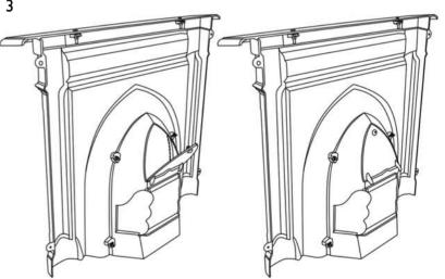
Rest the Damper Plate onto the grove on the back of the Fireplace Fascia.
