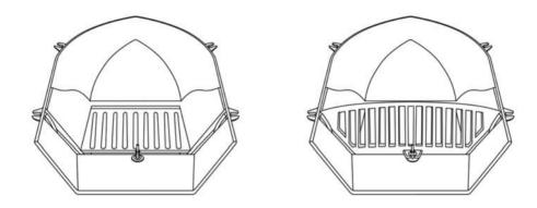
Lay Fireplace Fascia on back and insert the Firebrick and  $I \times M6$  Grub. Insert Grate into the groves on the Fireplace Back, passing the fixing lug over the M6 Stud. Secure in place with  $I \times M6$  Washer and  $I \times M6$  Bolt.
